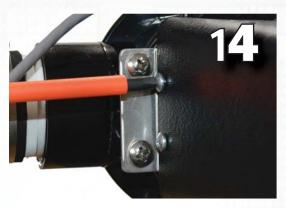
Reattach the pressure valve cover.
