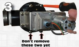
Carefully remove the top six screws, but temporarily leave the two on the bottom.
