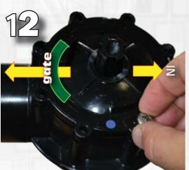
Slide the lid and gate assembly back into the Jandy valve housing. The raised "IN" stamp should be at 3 o'clock.
