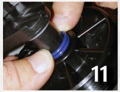
Use the gate shaft as a guide to seat the twin O-rings into the lid with your thumbs.
