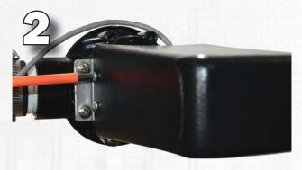
Remove the pressure valve cover by removing the two securing screws on the left side.
