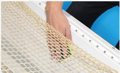
It's easier to unhook and rehook small sections of net to reach the various parts of the tub as needed.
