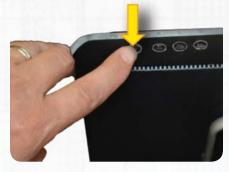
Hold the power button on the back of the touchscreen just until the screen blanks and then release the button.
