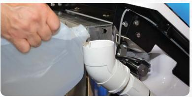
Gently pour in the distilled water and Defoamacide. Remove the fill tube.
