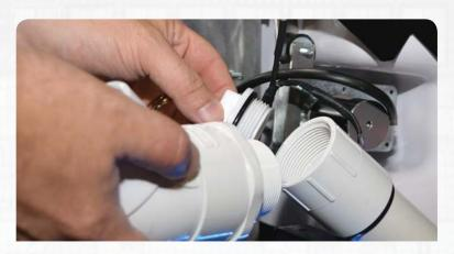
With all power removed from the lounge, unscrew the cap plug from the fill tube (no tools should be necessary) and screw-in the fill tube extension.
